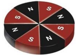
Sectors on One Surface Magnetised
